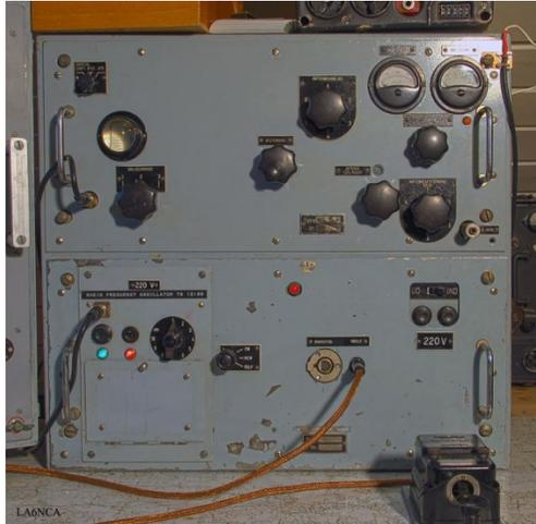
This radio was 40 watt, ran on 220 V AC had 3 vacuum tubes and weighed in at 163 pounds. You might wonder where you get 220 volts AC on a U-boat that runs on DC batteries. The radio room had a motor generator set that produced the required AC power.
