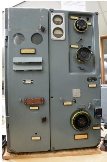
This rig was 19 x 30 x 18 inches and weighed a whopping 198 pounds! It operated on 7 vacuum tubes, produced 200 watt output and required 220 V AC power.
