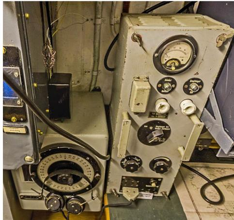
Operated from 300-600 kHz, 150 watt CW, had 3 vacuum tubes, again powered by 220 V AC, and weighed in at 24 pounds.
